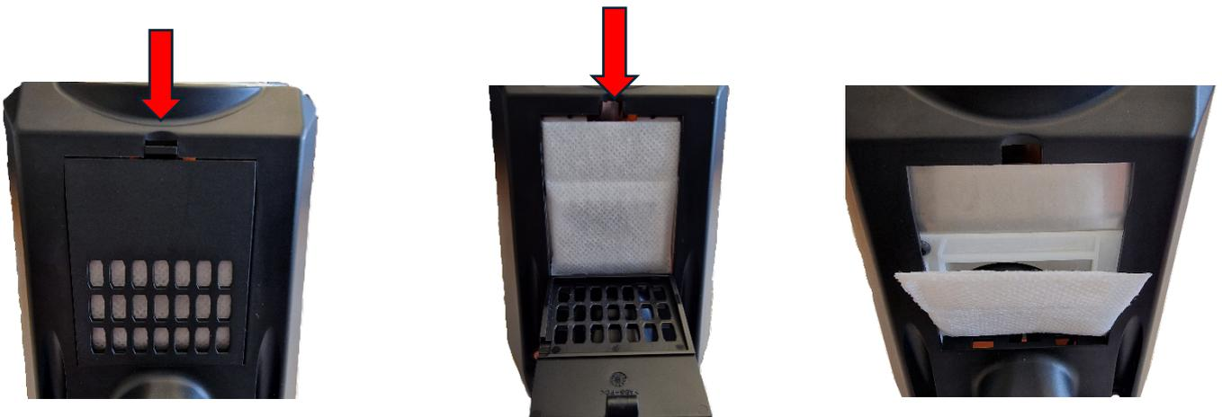
For older Flex V2 versions, it may happen that the filter flap still has the positioning hooks. Simply snip these off with a pair of side cutters.
