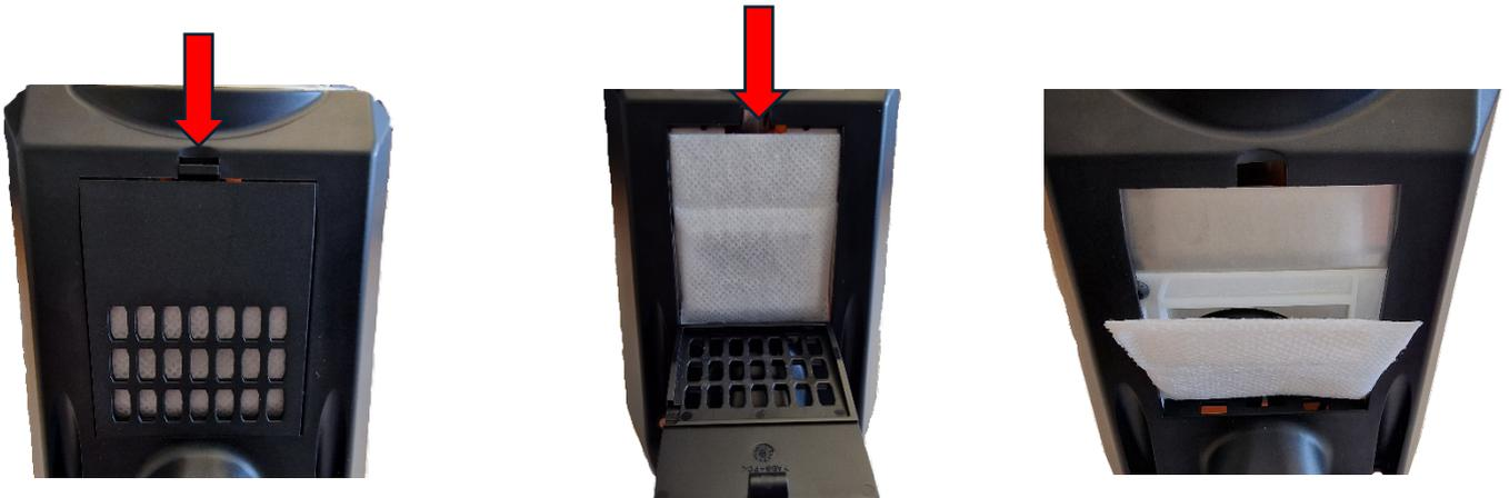
For older Flex V2 versions, it may happen that the filter flap still has the positioning hooks. Simply snip these off with a pair of side cutters.
