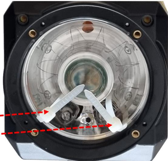
Use the two cable ties to carefully pull out the Bulb /
