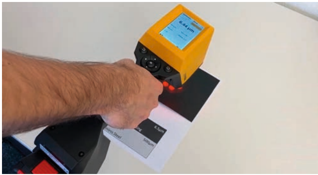
Figure 1 > Coating thickness measurement with the hand-held measuring device based on ATO technology.
