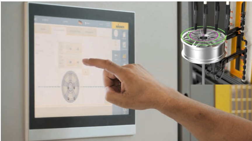
Figure 5 > The powder coating system, which has been developed specially for wheels, is configured and controlled via a touch screen.
