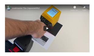
2 Video: coatmaster Flex measures the coating thickness of an e-coat on sheet metal accurately and precisely (test of repeatability) <a href="https://www.youtube.com/watch?v=45cOmm">https://www.youtube.com/watch?v=45cOmm</a> KZFDs
