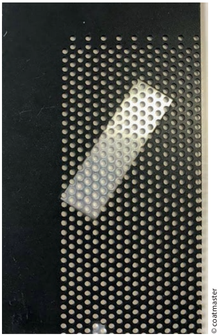
Figure 2 > Sample panel with perforated and non-perforated areas and bonded coating thickness disc.
