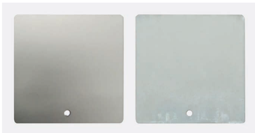
Figure 1 > Test panels with a coating thickness of 9 µm: without exposure (left) and after 1200 hours of the salt spray test in accordance with ISO 9227 (NSS) (right).
