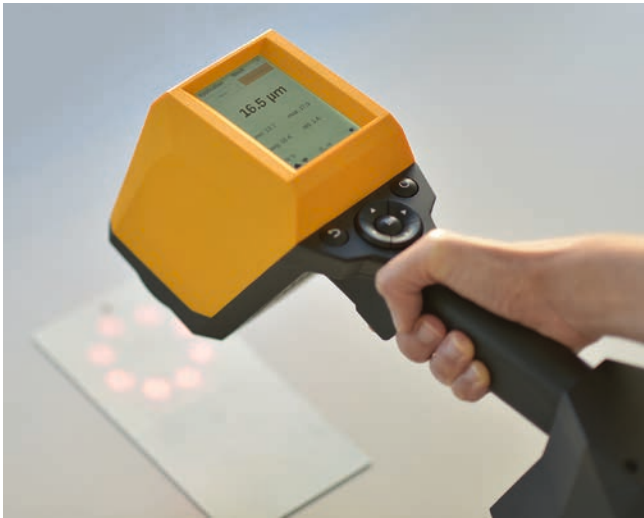
Figure 3 > Hand-held device for non-contact measurement of the thickness of wet and dry coatings.
