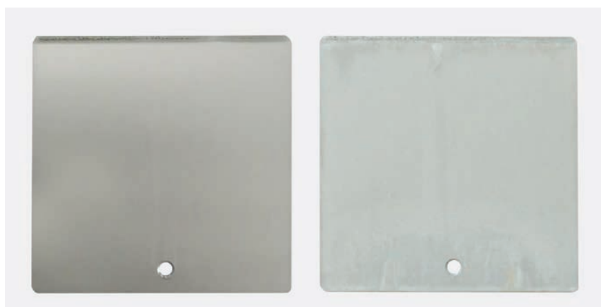
Figure 2 > Test panels with a coating thickness of 11 µm: without exposure (left) and after 2500 hours of the salt spray test in accordance with ISO 9227 (NSS) (right).
