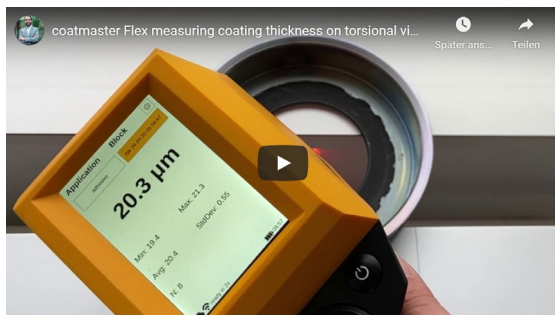
1 Video: Repetitive measurements using the coatmaster Flex on an adhesive agent coating on a flywheel of a torsional vibration damper. https://www.youtube.com/watch?v=zB7ZsbOIQc4
