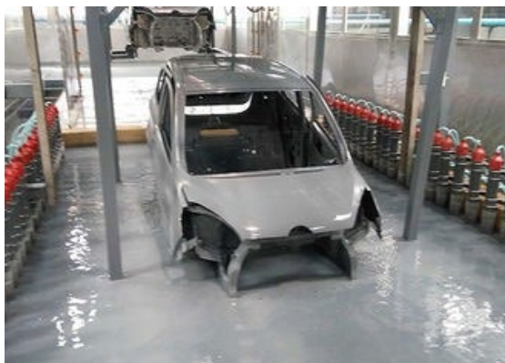
1 A car body immersed in a cathodic dip system.
