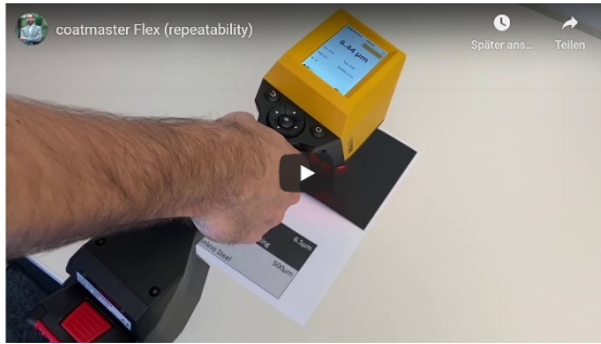
3 Video: coatmaster Flex measures the coating thickness of a cathodic-dip-coating on sheet metal (test of repeatability) https://www.youtube.com/watch?v=Ox1gkXl1RcY
