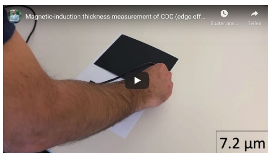
2 Video: Magnetic-induction thickness measurement of a cathodic-dip-coating on sheet metal (edge effects)
