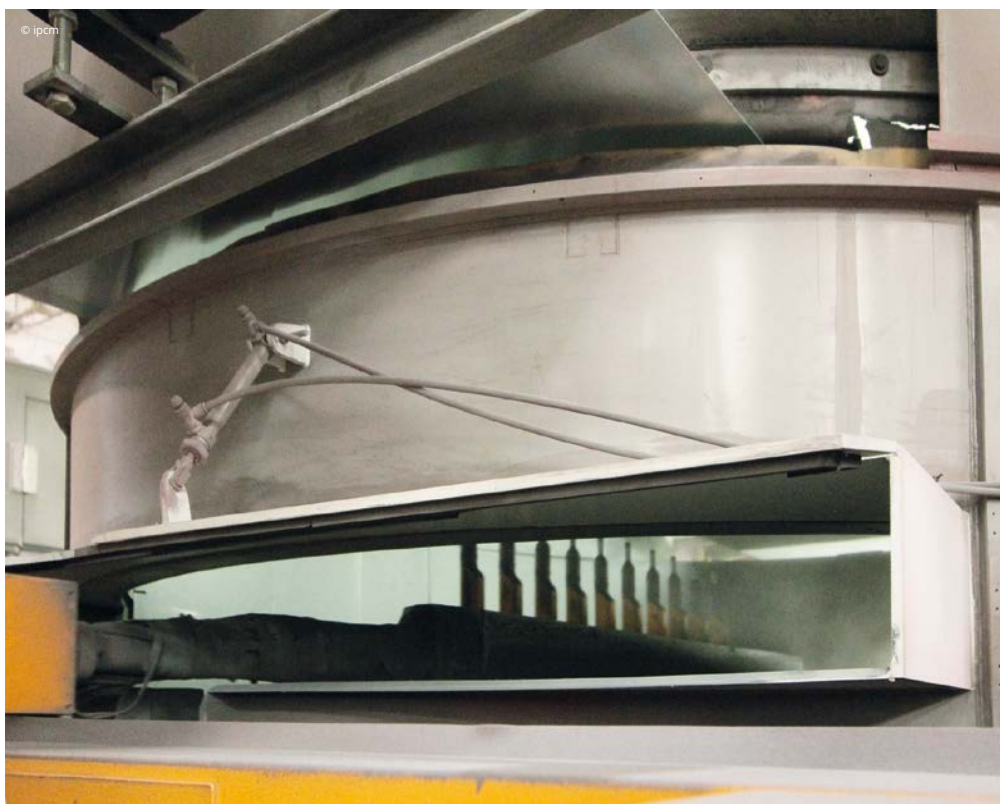
The detail of the coating guns mounted on the reciprocator.
