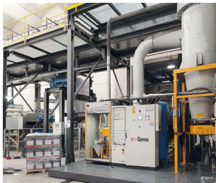
The powder management unit with an integrated ultrasonic sieve and dense phase powder transfer pumps.
