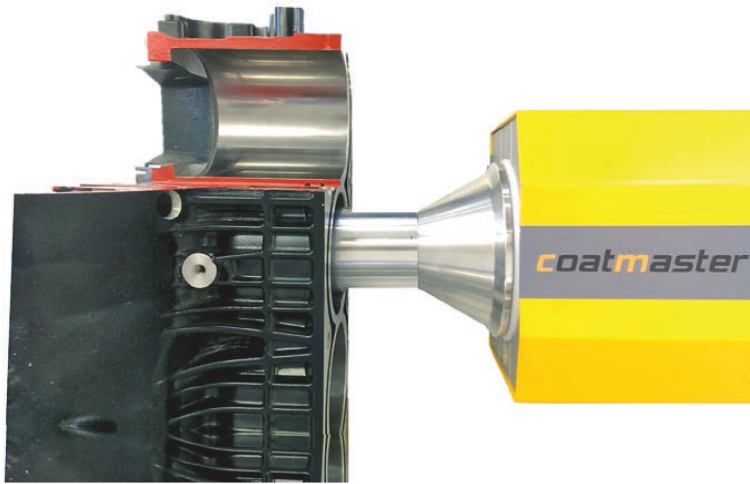
Figure 2 > For coating thickness measurement, the measuring optics are inserted into the cylinder bore (upper bore cut open). Thus, the coating thickness can be reliably measured at any position in the circumference and in the depth of the cylinder bore.
